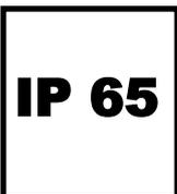
The IP rating is commonly expressed as **IP (Ingress Protection)** is followed by 2 numbers (i.e. 65) where the numbers define the fixture rating. The first number indicates the size of a particle that can enter the fixture. The second number indicates the extent of protection against water entering the fixture. An IP65 rating in this fixture indicates that dust particles can not enter the fixture. And there is protection against powerful water spray from entering the fixture from any direction.
