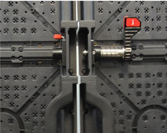
1. Latch has to be positioned in in the clockwise turning position were the red Open tap is visible.
