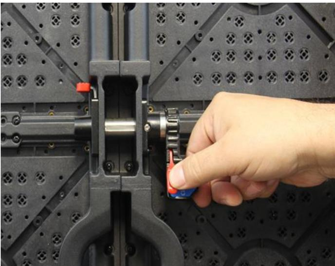
1. Press the red release trigger over the closed latch and hold down while at the same time turning the latch clockwise to loosen latch
