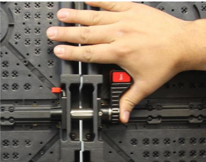
2. Push latch into the receiving latch position. Make sure the latch insert has passed the locking point and will not release if pulled back
